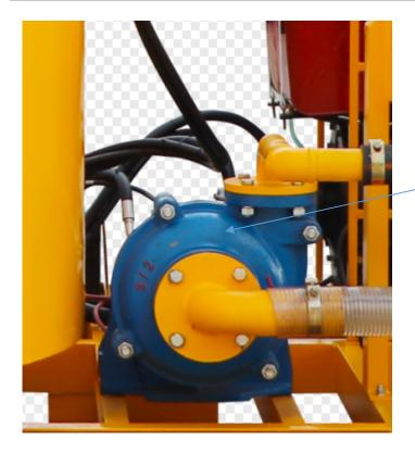
Heavy-duty slurry pump for recirculating and discharging
