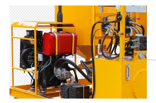
Diesel engine has strong power, paired with hydraulic system, the usage scenarios of the equipment are more flexible and diverse
